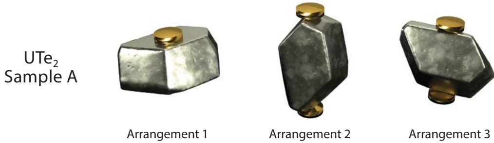
Figure F.1: UTe_2 sample A arrangements. The 3D model of UTe_2 sample A is shown in different arrangements between two piezoelectric transducers (gold). These different arrangements represent different ways we mounted the sample in the RUS setup to estimate the uncertainty due to the weight of the top lever on the sample. Arrangement 2 is the one chosen for the fit results in the main text in section 5.2 . Figure adapted from [43] .
